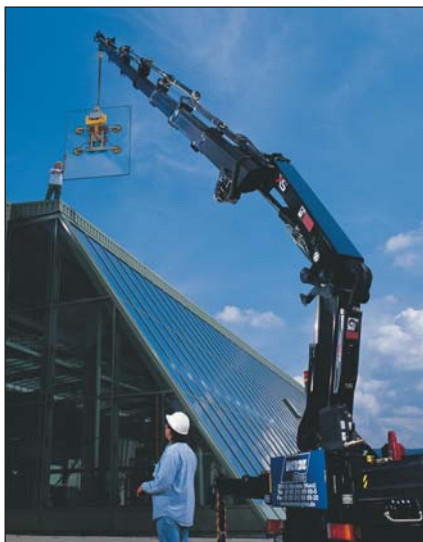
The new SSAB Domex 1200 hot-rolled, ultra-high-strength structural steel from strip offers crane manufacturers around the world new opportunities for producing strong crane booms.
