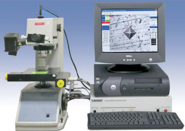
An automatic traverse Clemex microhardness system upgraded with a Newage C.A.M.S. computer and software.
