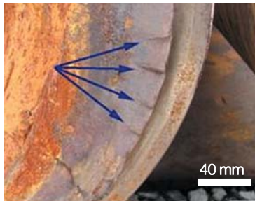
Fig. 5 — Ratcheting marks, indicated by the arrows, in a SAE 1045 shaft fractured by fatigue.
