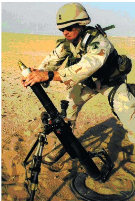
Fig. 1 — The flowformed mortar tube was live-fire tested at the Yuma Proving Grounds in Arizona by U.S. Army personnel.
