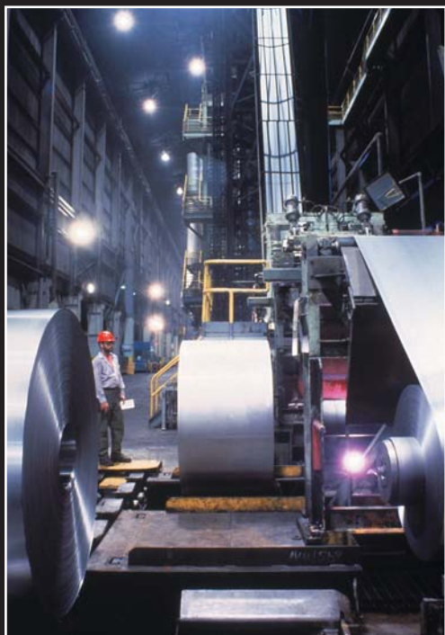
Continuous electrolytic tinning line at a U.S. Steel facility.
