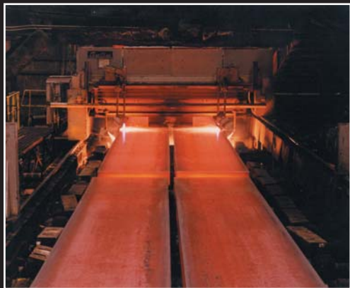
Continuous slab caster at a United States Steel facility.
