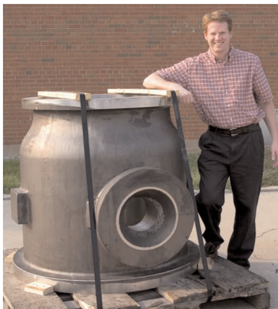
Fig. 1—Mike Pollard stands next to a prototype centrifugal casting of the end-cover for the Solar Turbines Mercury 50 recuperated gas turbine engine at the Caterpillar Technical Center. It was cast with DF8C-Plus steel by MetalTek International in 2005. An 8000-pound cast heat produced the 6700-pound component.
