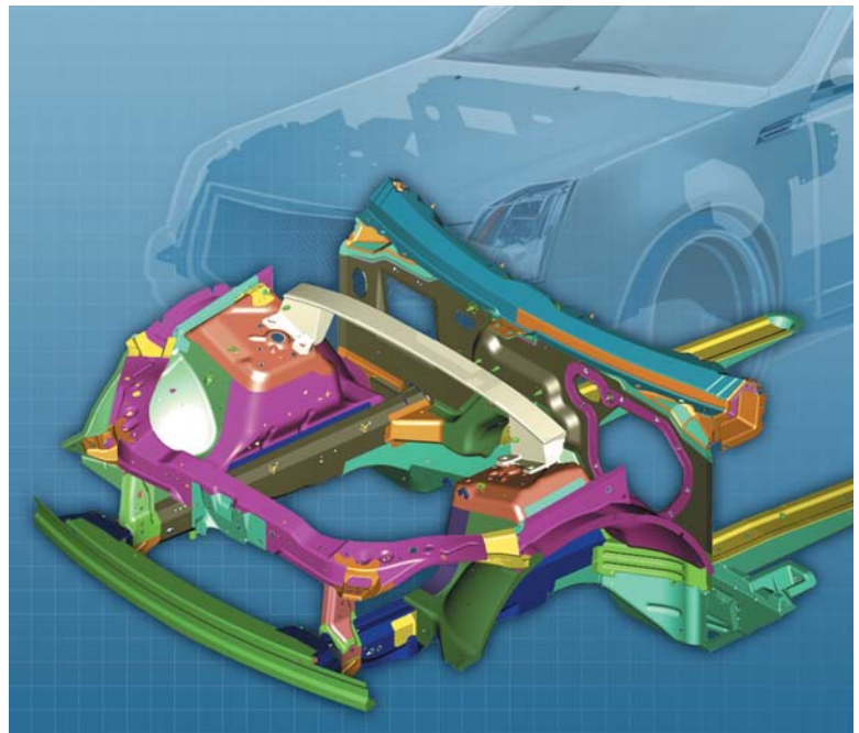
Fig. 1 — New alloys and processing methods for an economically feasible magnesium front end in magnesium-intensive vehicles are under development by engineering teams from Canada, China, and the United States.
