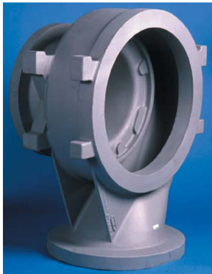
Fig. 2 — Wood patterns can be used to produce rammed graphite molds.
