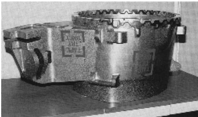
Fig. 2.2 Investment cast titanium transmission case for Osprey vertical take-off and landing aircraft
