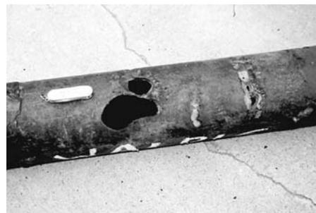
Fig. 5 Pipeline that experienced stray current corrosion caused by inverting the electrical leads to a cathodic protection rectifier
