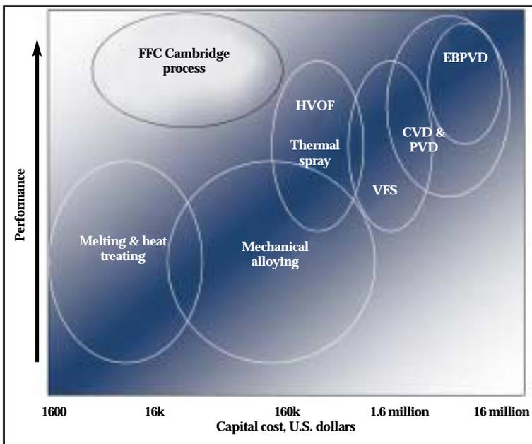
Fig. 3 — Performance and cost considerations for the FFC Cambridge Process and other alloying technologies.
