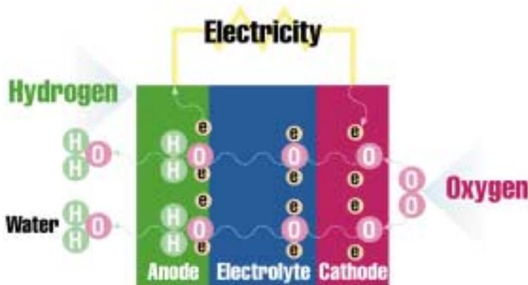
*Pacific Northwest National Laboratory is developing hydrogen-based solid oxide fuel cells (SOFC) for military applications, commercial power plants, distributed generation for residential and commercial use, and auxiliary power units for public and personal transportation. Also, SOFCs may be used for large-scale stationary power generation.*
