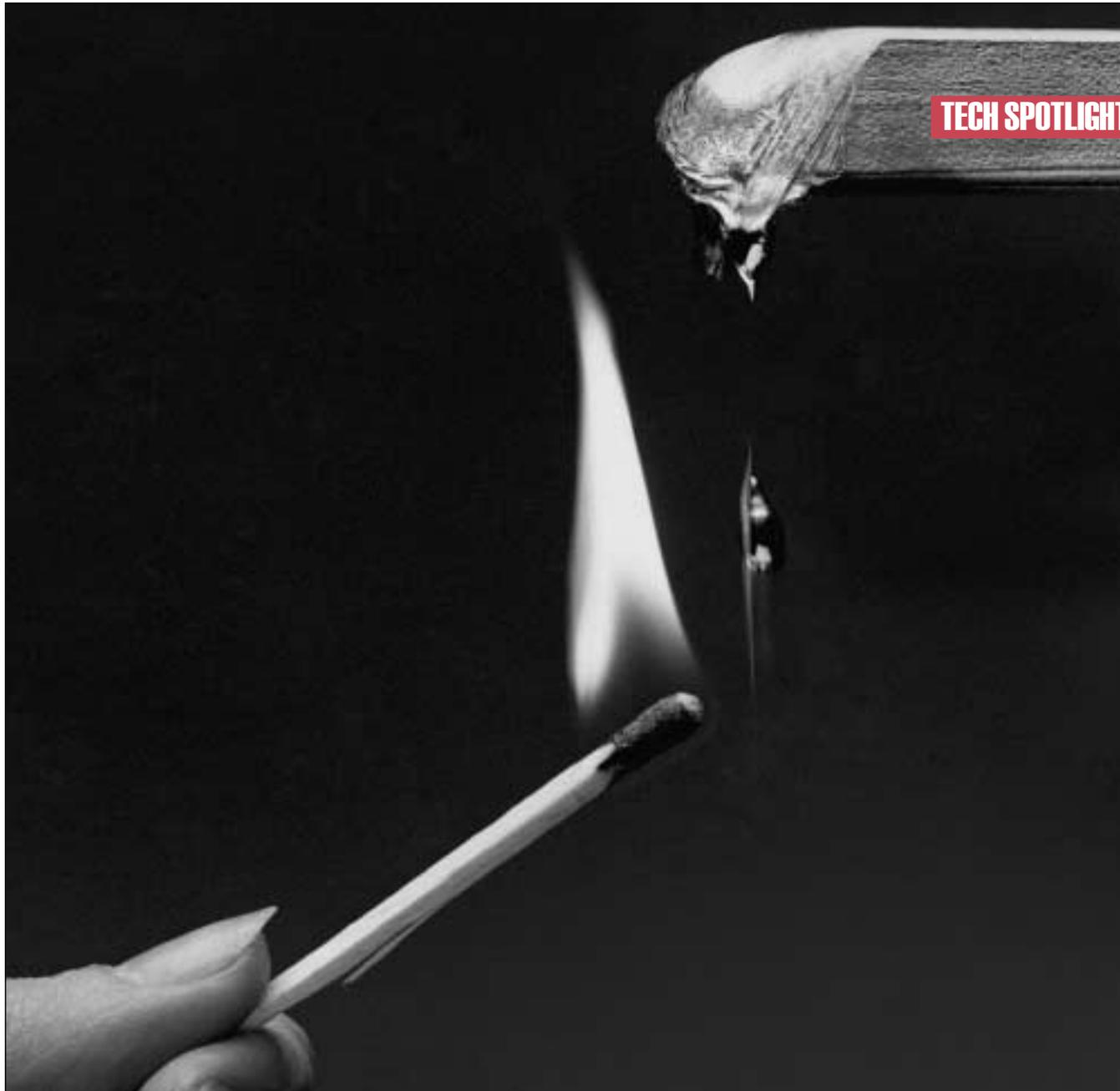
Fig. 1 — Pure indium melts at a temperature of  $156.7^{\circ}\text{C}$  ( $314^{\circ}\text{F}$ ). Image courtesy Indium Corp. of America.
