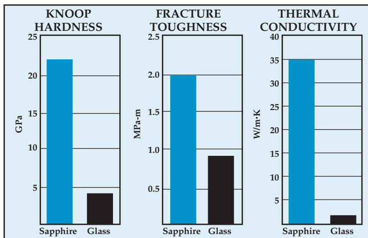
Fig. 3 — These graphs compare selected material properties of glass and sapphire. They show the superior properties of sapphire.
