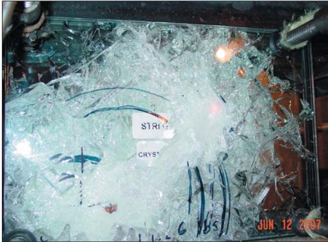
Fig. 4 — Front Panel, Sapphire Transparent Armor system (229mm x 330mm) is shown defeating four-shot multi-hit 7.62 x 39 API-BZ, Full STANAG Level 2. Full STANAG Level 2 Testing of four shots is considered difficult due to the spacing relative to shots #1 and #2, and #3 and #4.
