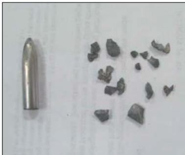
Fig. 2 — These images show the 7.62x54R B32 API hard projectile core before (left) and after impact (right) on sapphire strike face. Note the total destruction of the hard projectile core after contact with the Sapphire Transparent Armor system.
