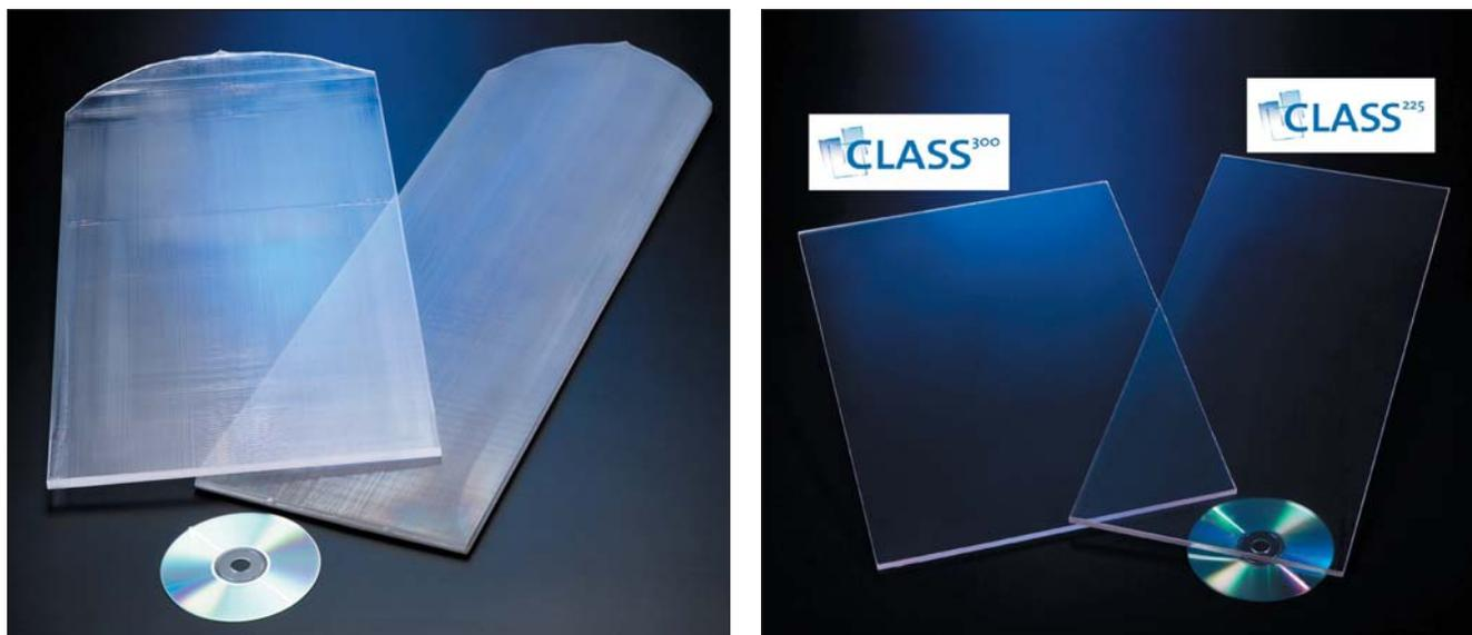
Fig. 1 — These are CLASS<sup>300</sup> and CLASS<sup>225</sup> (Clear Large Aperture Sapphire Sheet) as grown (left) and after polishing (right).
