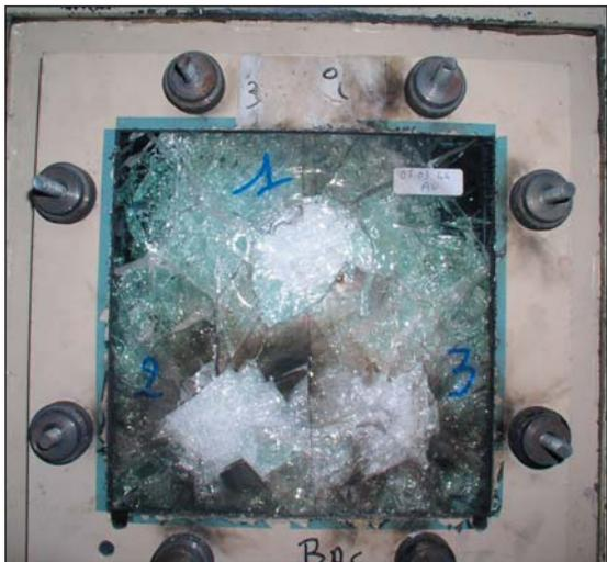
Fig. 6 — Sapphire Transparent Armor system (305 mm x 305 mm) is shown after defeating multi-hit 7.62 x 54R B32 API.
