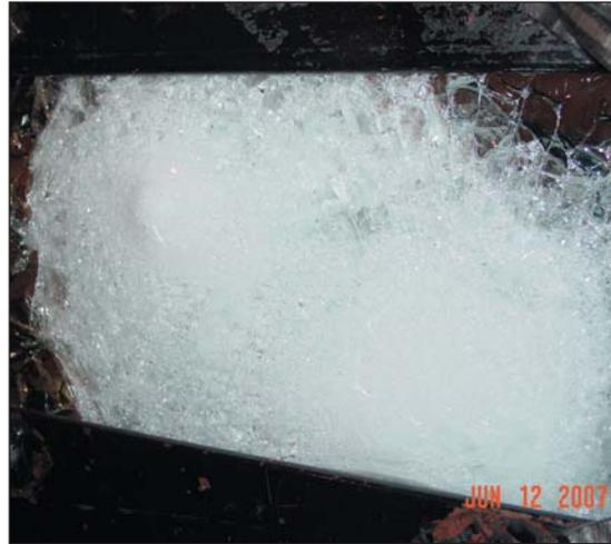
Fig. 5 — The Rear Panel, Sapphire Transparent Armor system (229 mm x 330 mm) is shown defeating four-shot multi-hit 7.62 x 39 API-BZ, Full STANAG Level 2.
