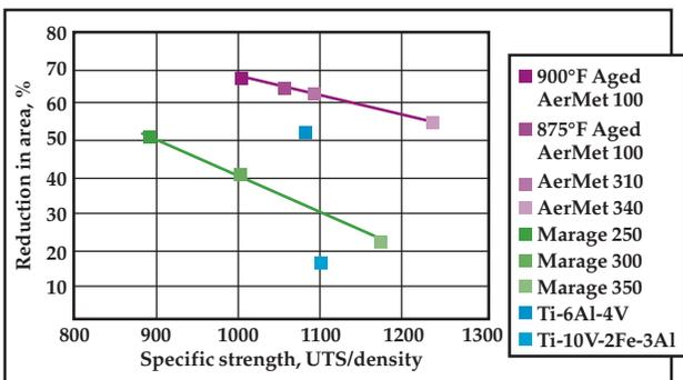
Fig. 5 — Reduction in area vs. specific strength.
