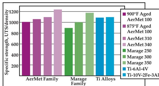
Fig. 2 — Specific strength comparison.
