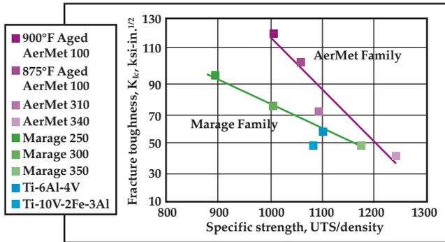
Fig. 7 — Fracture toughness vs. specific strength.
