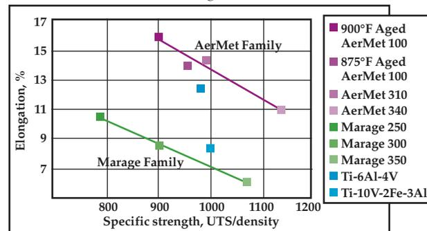
Fig. 4 — Elongation vs. specific strength.
