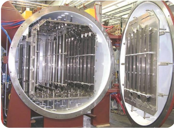
Fig. 2 — Batch vacuum aluminum brazing furnace.
