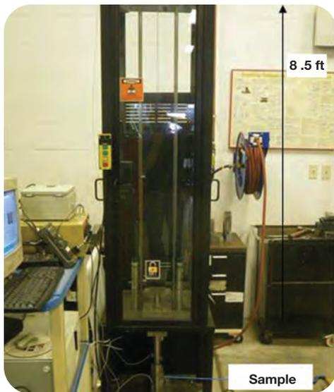
**Fig. 8** — Drop tower for high speed sample testing.
