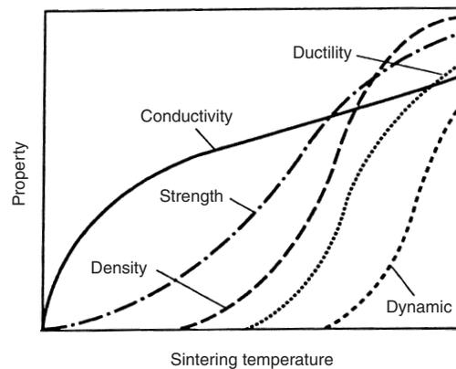
**Fig. 5.2** Variation in compact properties with degree of sintering, as represented by sintering temperature. Source: Ref 2. Reprinted with permission from MPIF, Metal Powder Industries Federation, Princeton, NJ
