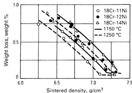
**Fig. 5.4** Relationship between sintered density and weight decrease of three austenitic stainless steels in 40% HNO<sub>3</sub>. Source: Ref 7. Reprinted with permission from MPIF, Metal Powder Industries Federation, Princeton, NJ
