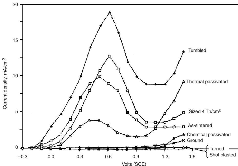
Fig. 5.12 Potentiodynamic curves of 316L stainless steels as a function of surface finishing treatment. Reprinted with permission from MPIF, Metal Powder Industries Federation, Princeton, NJ
