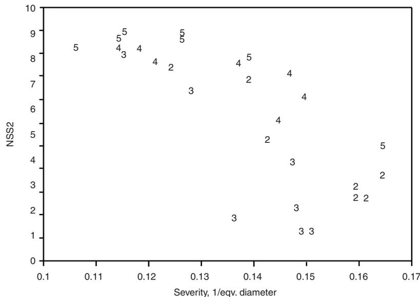
Fig. 5.9 Visual rating after 1500 h salt spray test versus severity value calculated as the reciprocal of average pore diameter. Reprinted with permission from MPIF, Metal Powder Industries Federation, Princeton, NJ
