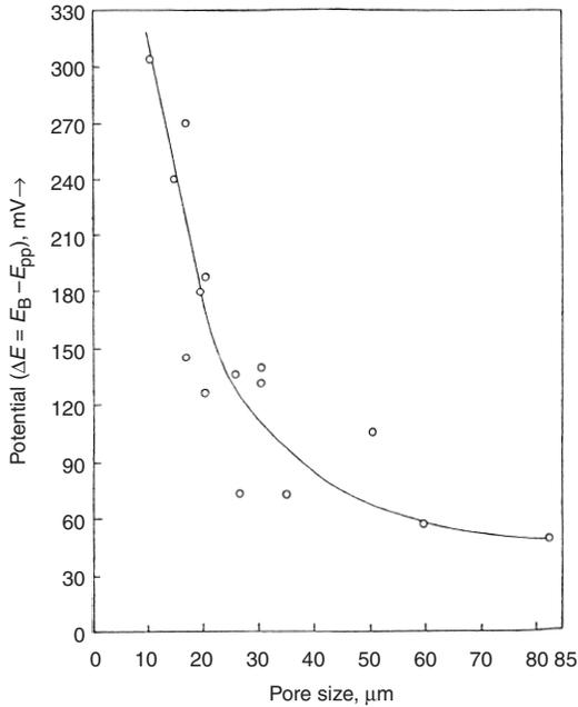
**Fig. 5.6** Effect of pore size on size of hysteresis ( $E$ ) for sintered 316L in 3% NaCl (27 °C, or 81 °F). Source: Ref 14. © NACE International 1989
