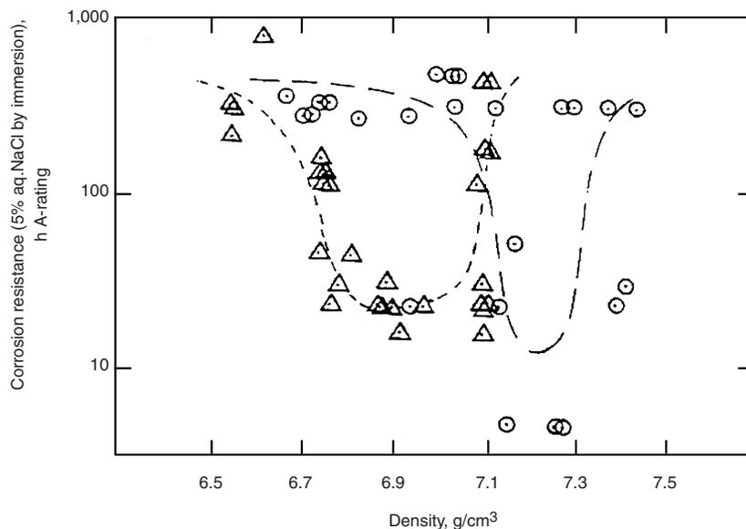
**Fig. 5.5** Effect of density on corrosion resistance of 316L parts.  $\Delta$ , pressed and sintered only;  $\circ$ , pressed, sintered, re-pressed, and annealed. Source: Ref 13. Reprinted with permission from MPIF, Metal Powder Industries Federation, Princeton, NJ
