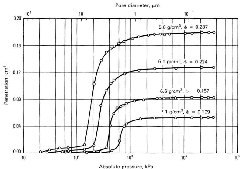
**Fig. 5.11** Mercury porosimetry curves of sintered steel parts of varying densities. Green skeletons were sintered at 1093 °C (2000 °F) for 20 min. Total porosity ( $\phi$ ) is determined from sample weight and dimensions. Source: Ref 21
