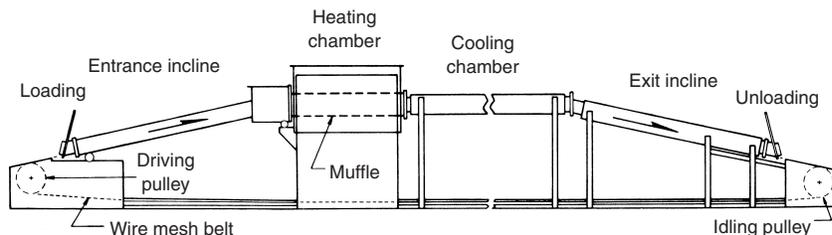
**Fig. 5.1** Schematic of a humpback mesh belt furnace. Source: Ref 1. Reprinted with permission from MPIF, Metal Powder Industries Federation, Princeton, NJ
