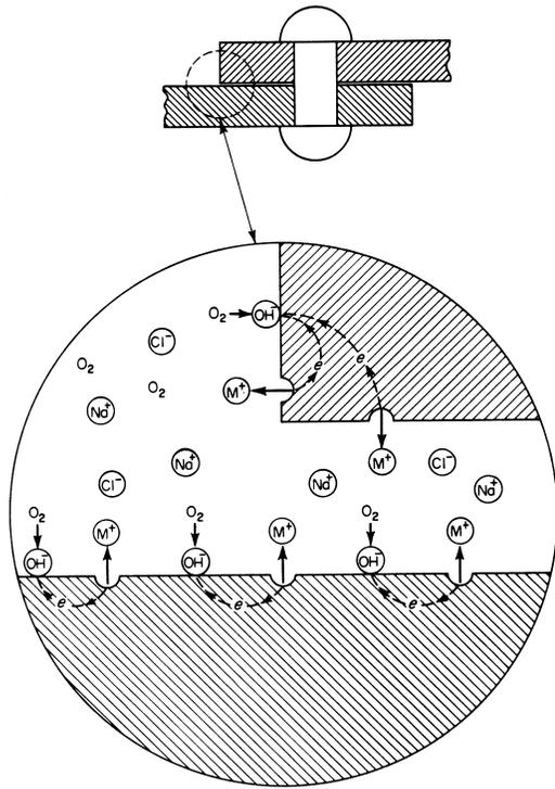
**Fig. 5.7** Crevice corrosion mechanism—initial stage. Source: Ref 15. Reprinted with permission, Fontana, *Corrosion Engineering*, 2d ed. © The McGraw-Hill Companies, Inc., 1978
