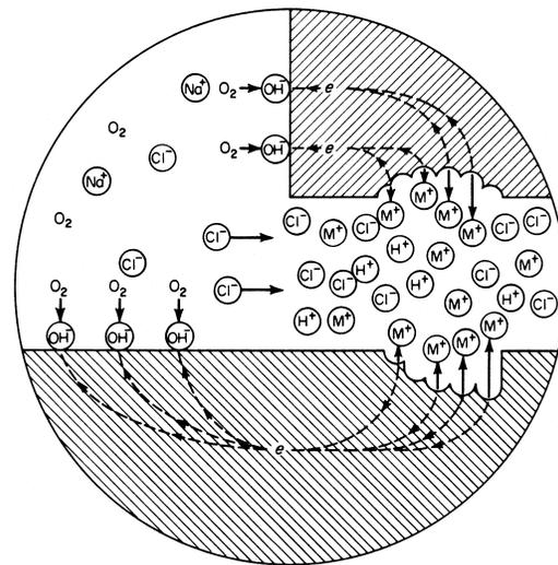
**Fig. 5.8** Crevice corrosion mechanism—later stage. Source: Ref 16. Reprinted with permission from MPIF, Metal Powder Industries Federation, Princeton, NJ
