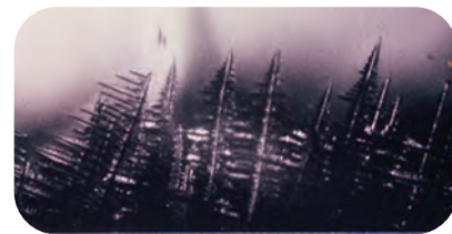
Fig. 3 — Trepanned single crystal ingot showing “freckle” trails.
