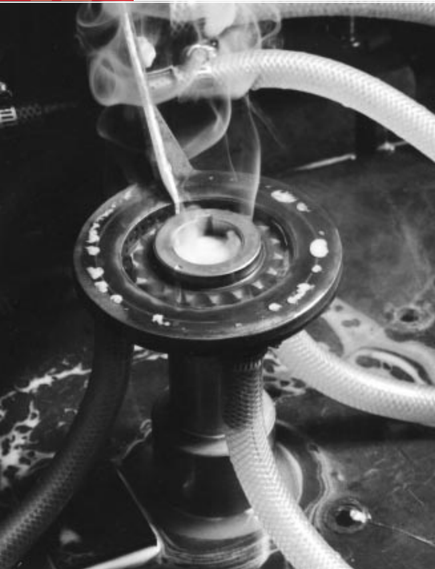
Powder Metal automotive sprockets being induction hardened on a lift/rotate work station.
