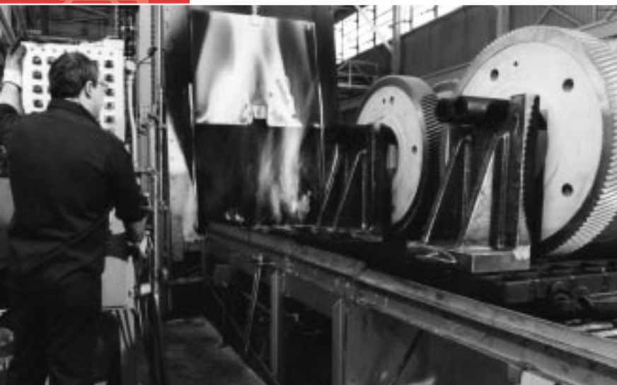
Gears suspended from the bore vertically to minimize distortion. Parts are masked with stop-off paint to prevent carburization of areas requiring subsequent machining after heat treat.
