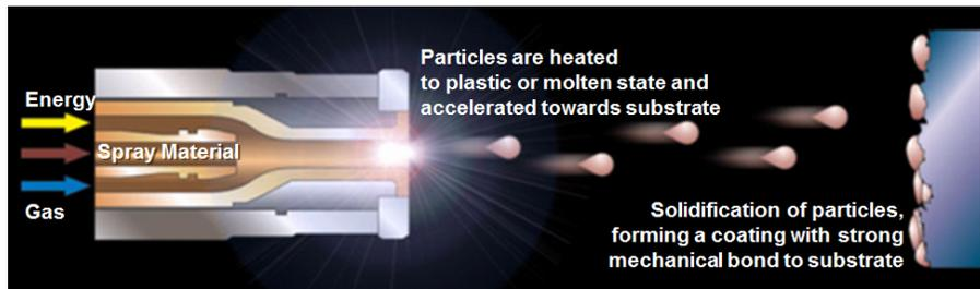
Figure 2b: Principle of Thermal Spray Coatings
