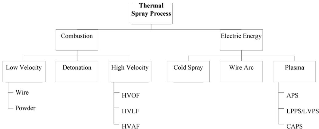
Figure 3a: Types of Thermal Spray Processes (HVOF: High Velocity Oxy-Fuel; HVLf: High Velocity Liquid-Fuel; HVAF: High Velocity Air-Fuel; APS: Air Plasma Spray; LPPS/LVPS: Low Pressure Plasma Spray/ Low Vacuum Plasma Spray; CAPS: Controlled Atmospheric Plasma Spray)
