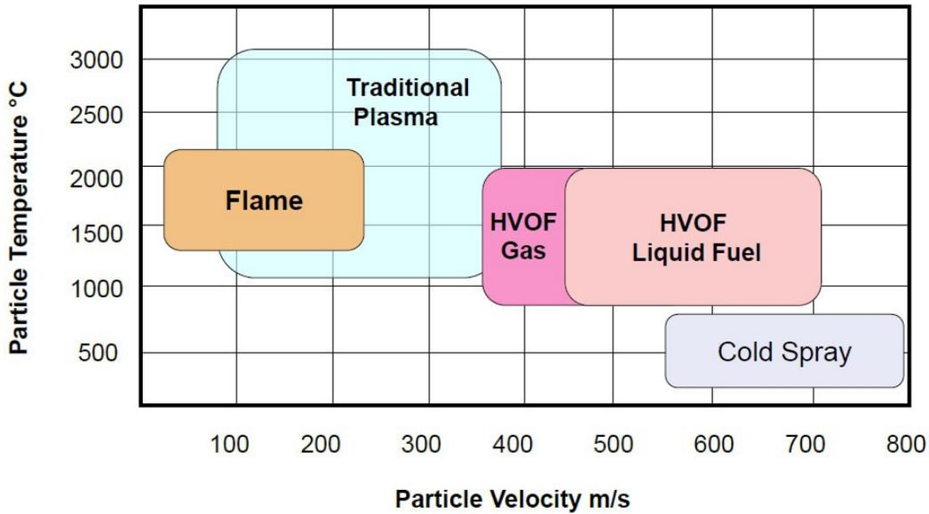
Figure 4a: Overview of Particle Temperature versus Particle Velocity for Different Processes
