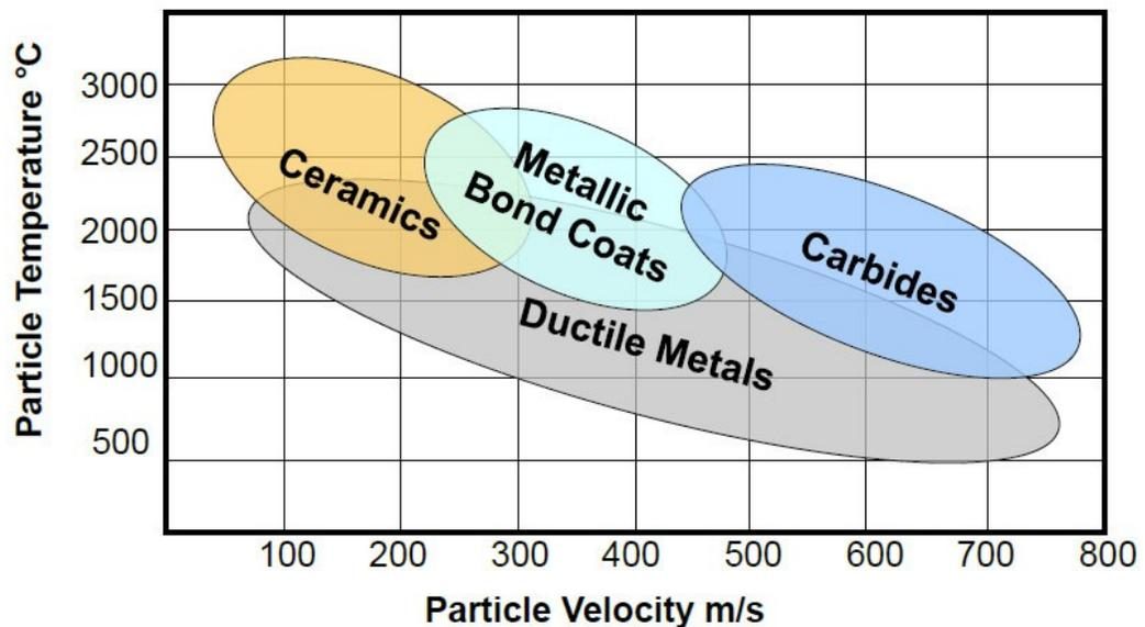
Figure 4b: Overview of particle temperature versus particle velocity for different materials systems
