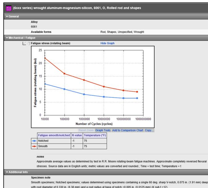
Figure 8: The Structural Materials Data Demonstration Repository and Database includes mechanical property data such as fatigue strength versus number of cycles to failure.
