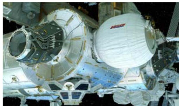
**Fig. 2:** The BEAM module will be attached to the rear port of the space station's Node 3. After installation, the BEAM expands to roughly 13-foot-long and 10.5 feet in diameter. Credits: Bigelow Aerospace, LLC
